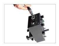
CAUTION: The power specification we have provided is as per 12volt. For this, we provide a 12volt/3ampere regulated power adapter. In case you use a voltage higher than 12V, it will affect the performance and life of the motor, and there is a high risk of the motor getting damaged.
