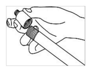
Screw-in the adapter mounted on the blimp with the adapter on the boom pole.
