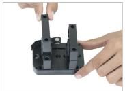
• Remove the screw bush by removing the handlebar.
