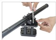
• Remove the 4 X bolt, as shown in the image.
