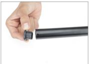
Loosen the bolts of the Flycam swivel with the help of a 4mm Allen key and insert the rod.
