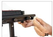
Open the lever and remove Quick Release Plate from Adapter (Part-6). Then attach it with your camera with the help of screw driver. Insert your camera setup into the Adapter and tighten the lever back.
