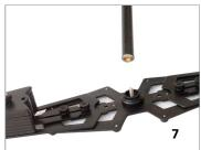
**NOTE:** The adjustment knob should only be tightened by hand. Do not over-tighten it as it could cause thread stripping.
