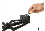
On base platform (Part-2) is made by loosening the retaining screws and moving counterweight plates (Part-4) closer to or farther away from post and then re-tightening. You will probably need to adjust and re-adjust the horizontal position to achieve optimum performance.
