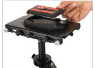
Now attach the quick release adapter to the bottom of the camera (Not Included) and tighten the bolts using the screw driver.
