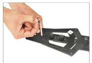
• Similarly, follow the same procedure to insert each M6 screw into the base platform.
