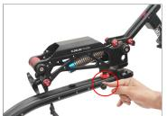
To fix the placid arm at its appropriate position, attach one side of the safety shock cord to a knob on the placid arm. Then, drag the other side of the elastic cord across the flowline support arm, and attach it to the knob on the other side of the placid arm.
