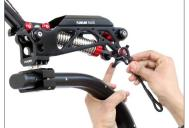
Using an allen key, pull the mounting bracket of the placid arm out of the flowline support arm and remove the cord from the bracket. Make sure it comes out precisely through the hole in the placid arm.
