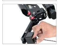
To remove the placid arm from its position, unscrew one side of the safety elastic cord from the plaid arm's knob. Then, pull the other side of the elastic cord out from the flowline support arm.
