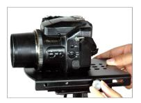
The many slots on the head and bottom plates allow you to adjust the X & Y axis for perfect balance easily. Once achieved, tighten the knobs to secure. Further 'fine tuning' will probably be required..
