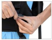
When folding Flycam Flowline, always make sure to put the upper part of Support Arm inside hip/waist belt and fasten buckle at the hip/waist belt. This will prevent Suspension Line from wearing.
