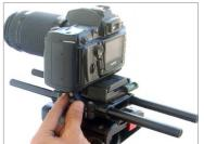
Attach both Cage Brackets with rods and tighten the knobs to secure them appropriately.
