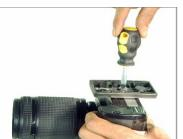
Now mount camera with Quick Release Plate on the Camera Base and tighten knob properly to secure it.
