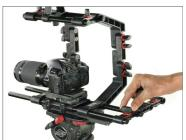
Then insert 300mm male threaded rods into the Straight Bracket and tighten knob to properly lock them.
