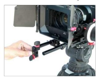
Now slide-in one 300mm female rod through it in order to attach Handles and tighten knobs to secure the adapters and rod properly.
