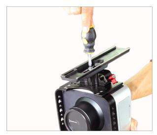
• Now mount Cage onto any standard tripod and secure it.
