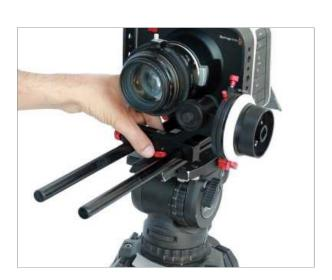
Now attach Matte Box to the front of rods, align knicker with lens barrel and tighten the knot.
