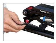
Now mount your camera setup on hook of Flowline and tighten the knob to secure it properly.
