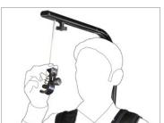
Attach camera to hook and tighten with provided knob to ensure slip-free connection.
