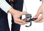
• Secure the Placid on Flowline Arm with provided tie to ensure slip-free connection.
