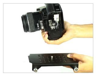
**Note:** Do not over tighten this adjustment as it can break the threaded insert.
