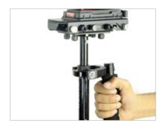
For shots that require framing the camera up, down or sideways, hold the handle firmly at bottom.
