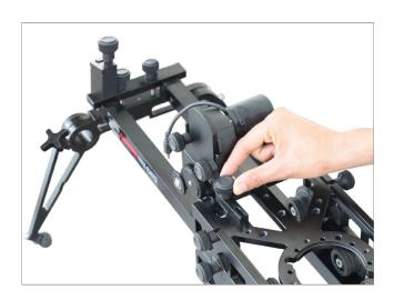
Now, Adjust the motor part as shown in the image in order to attach the belt on to the pulley.
