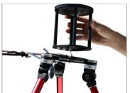
• Re-insert the bolts and tighten with Allen key properly.
