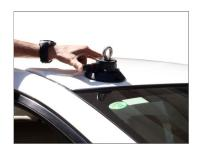
Attach one end of Rope with metal Hooks to camera mounting platform and another end to Metal loop of Suction cup. Tighten the Rope properly.
