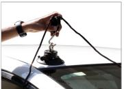
• Now loosen the four Allen bolts on Camera platform, align 100mm bowl with it.
