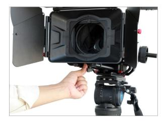
Align knicker to Matte Box, mount it over the front lens and tighten its thread.
