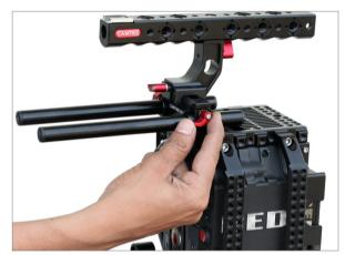
• Similarly, insert the two 300mm aluminium rods into 15mm rod adapter of Base Plate and tighten the knob correctly.
