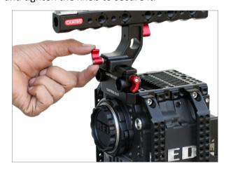
• Insert the two 200mm aluminium rods into 15mm adapter holes on top of the Cage and tighten the knob properly.
