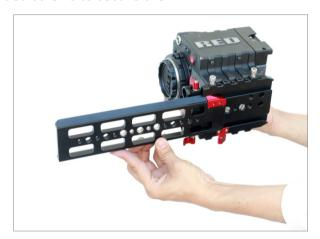
Now attach Quick Release Plate to Dovetail Plate and mount it on tripod. Tighten the knobs to secure it well.
