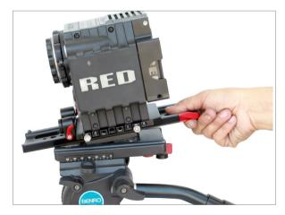
Attach the four Cage Brackets to Base Plate and fix them tightly using allen key. Then mount
