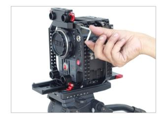
• Now slide-in Top Handle on 15mm rod adapter and tighten the knob to secure it.
