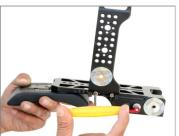
Attach the top plate with lens support side bracket and then insert two 200mm rods into 15mm rod adapter. Tighten the knob to secure it.
