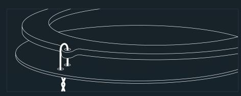
Place a bead of RetroRubber sealant in channel of headlight housing as shown. Fill the majority of the channel to ensure it sufficiently holds the front lens once re-installed.
