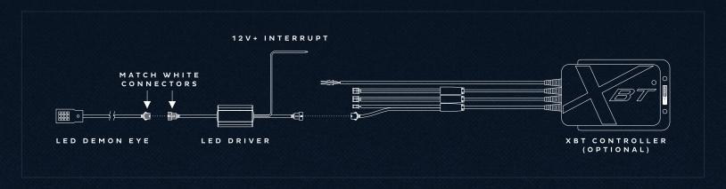
NOTE: The 12V+ Interrupt Wire needs to be tapped or spliced into a 12V+ lead that has power when the HID bulb of the projector is illuminated to deactivate power going to the LED Demon Eye.
