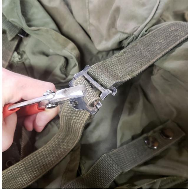
2. Once the rearmost bar on the ladderlock is broken, move the cutting pliers to the next highest bar and bend until failure.
