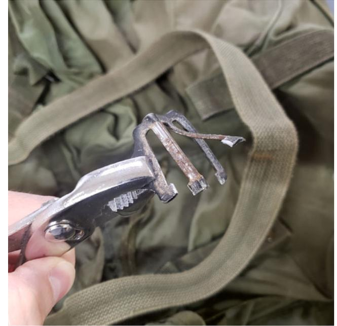
3. Repeat step 2 on the remaining ladderlock bar, freeing the vertical compression strap from the ladderlock. Repeat steps 1-3 on the second vertical compression strap ladderlock.
