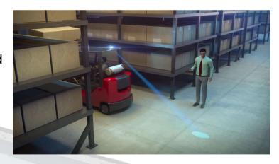
The blue safety spotter light can be installed on the front or the back of any forklift, sweeper or other piece of industrial equipment.
