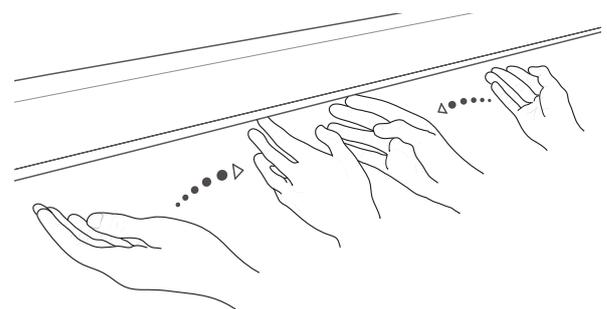
By moving 2 hands away from each other under the sensor strip, you can make the beam wider.
