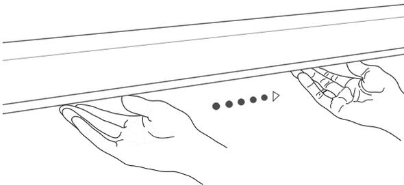
Another way to move the light beam is to hold your hand at the place under the sensor where you want to move the light beam. The light beam will then move towards your hand.
