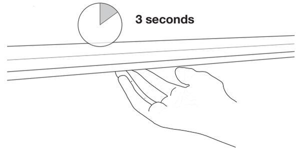
By moving your hand under the sensor, you "scroll" through the available colours. You can scroll forward and backward by moving the hand either from left to right or right to left underneath the sensor.
