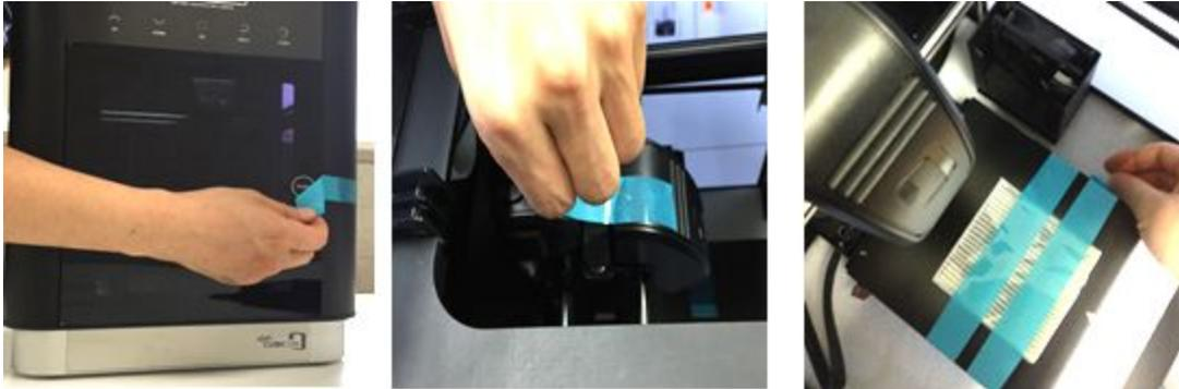
④ Remove extruder fixing straps (Cable Tie) –Remove fixing straps on the both side of the extruder by cutting them with scissors.
