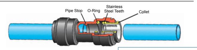
TO INSTALL PIPE/TUBE: Simply push the pipe in until it is seated firmly. Ensure the end of the pipe is square with no burrs. Push LOCKING CLIP into place (if applicable).
