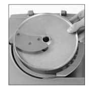
Next fit the appropriate slicing disc and rotate in a clockwise direction to check that it is correctly positioned.
