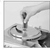
4 Position the automatic hopper on the motor base. The fastening hook is now facing you on your right.
