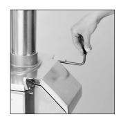
2 Slip the hinge pin into the locations provided at the back of the motor base. The locking handle should now be facing you, on the right.
