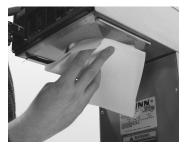
Use a clean damp cloth rinsed in mild, non-abrasive detergent to clean the sprayhead panel.
