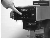
Place the "ON/OFF" switch in the 7. "ON" upper position.
