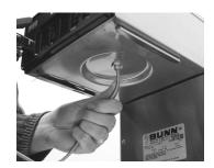
5. With the sprayhead removed, insert a deliming spring into the sprayhead tube until approximately two inches of the spring remain visible. Saw back and forth five or six times to loosen any lime deposits.
