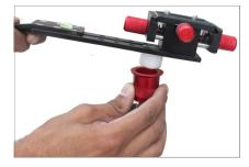
Now loosen the red knob as shown in the image, remove the camera mounting plate and secure your camera on it with the help of screw driver.
