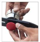
• Take the accessory mounting plate adapter & knob, attach accessory mount plate to stabilizer with the help of adapter and knob. Tighten it properly to secure.
