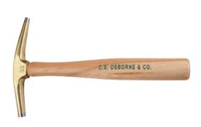
Solid head of bright bronze. Steel tipped at one end for permanent magnet and at the other for hammering. Balanced design, lacquered hickory handle. Replacement handles are also available **Osborne No. 33-H** UPC No. 56046.
