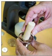
3.- Holding the die use the wood dowel to push in the shell.
