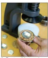
2.- Turn top of the two piece die. Place the cut material on the die, then center the shell on top of the material as shown.
