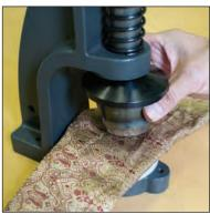
Place material on the nylon block. Lay cutter on material.
