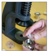
Lay wire eye on the bottom die with the loop facing down.
