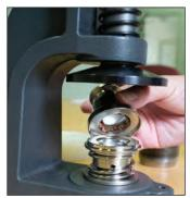
Place the two piece die together on the machine. Lock in the bottom piece die with the Allen wrench key provided.
