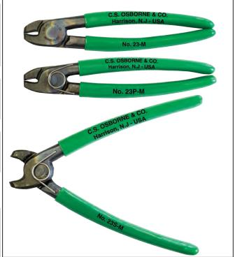
Tension type hog ring pliers. <u>The joint is held by a bolt, nut and tension washer;</u> this keeps the joint from freezing and helps hold the hog ring when pliers are laid down.
