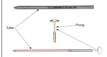
Prong is inserted into hollow end of needle. Needle is pushed through construction and withdrawn, leaving prong extended.
