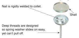
THREADED NAILS (For use with Spring Washer) When anchored with a spring lock washer, the Threaded Nail is a fast, positive, alternative to prong tufting. Just insert the nail through the upholstered construction and fasten in on the back with a spring washer.
