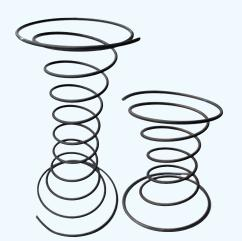
Open ended, 9 gauge. Upholstery springs are ideal for 8-way hand tied seating. Available in sizes from 5" to 10" height. Made of high carbon spring wire and heat treated for resilience. Sold in bundles of 25 lbs/bundle. Data in table below is approximate and not exact.
