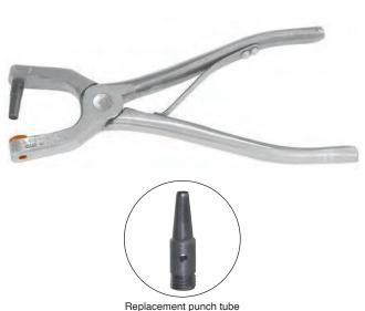
Forged steel frame. Highly polished. Fitted with replaceable screw tubes. Copper anvil. The throat distance from the cutting tube to the back of jaw is 1 1/2". Made in sizes 000 to 10. Weight each 12 oz.
