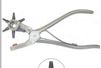
Six tube punch made with tubes 1, 2, 3, 4, 5, 6 or 0, 1, 2, 3, 5 & 7. This punch is the best Revolving Punch made. The frame is made of forged steel, highly polished. Cutting tubes are turned from special carbon tool steel and threaded to allow easy replacement. Copper anvil. Each tube is individually hardened. The throat distance from the cutting tube to the back of jaw is 1 1/4". Weight each is 15 oz. Size 1-6 provided unless specified otherwise.
