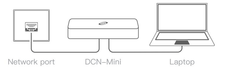
3. After hooking up the Ethernet cables, plug in the power cable to the Deeper Connect Mini. The devic will
