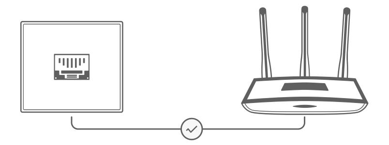
Do not power on the device . Connect the Ethernet cables to your Deeper Connect Mini by selecting and following a setup method (A, B or C) according to your network environment:
