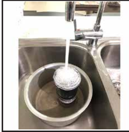
2. Wash the filter under running water for approximately 10 min or till it stop leaking black natural colour from the Activated Charcoal
