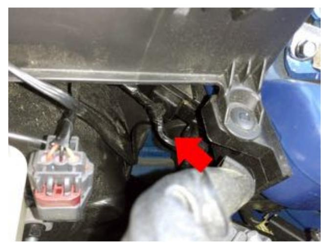
Route the cable across the cowl tucking it under the rubber grommet and plug it in to the 2 position matching connector near the JB4 control box. The latch on the connector must line up with the clip for CANbus to operate.
