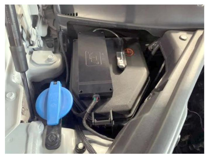
The optional OBDII cable unlocks full CANbus control for the most advanced tuning and logging features and is strongly suggested. The cable can be routed the "quick" way through the door jamb or the "clean" way through the firewall detailed below.
