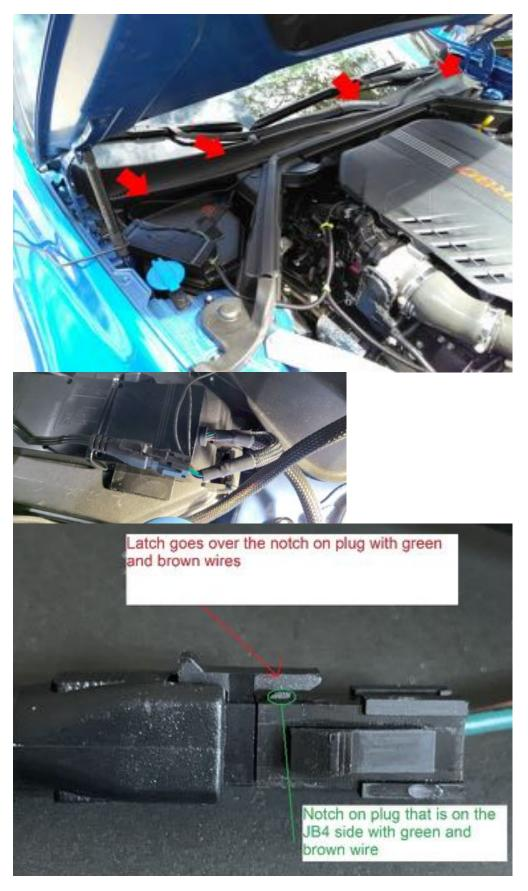
The JB4 includes optional black fuel control wires giving the JB4 the ability to directly change the air/fuel ratio. The factory tuning runs in the 10:1 range and leaning that out to 11.5:1 has proven to be worth significant power at higher engine speed. Note these are preinstalled on the JB4 harness now so only need to be attached to the o2 sensor signal wire to enable using the included posi-taps or our optional fuel harness adapters.
