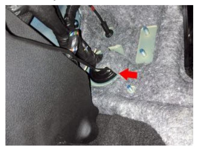
Remove the brake booster cover by popping up the 3 plastic locks that hold it down, reach down and pull the OBDII wire up.
