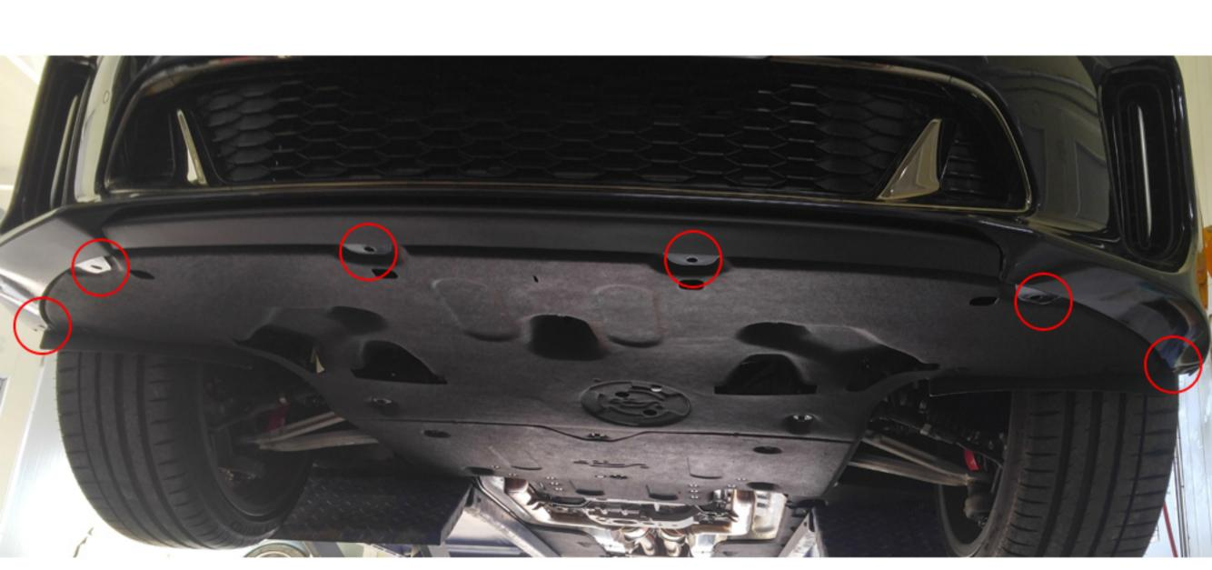
Remove the factory keys/pins from the places circled in RED
