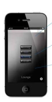
Individual lighting levels can easily be adjusted then saved to a button to be recalled at a later date. These settings are then saved to a local control panel within the room alowing editability of the system lighting levels.
