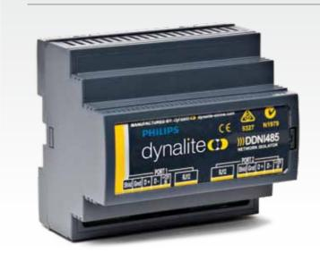
The Philips Dynalite DDNI485 is designed for cost-effective optical isolation of DyNet RS485 networks. The two opto-isolated RS485 ports enable the DDNI485 to implement a trunk and spur topology, with each spur being electrically isolated from the others so a fault in one section of the network will be contained. It is a "passive" device that does not require programming.
