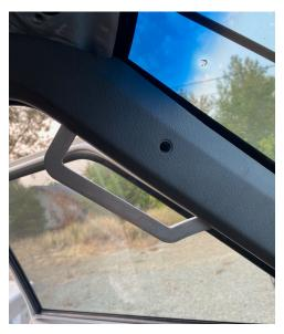
4. Using these marks, cut your trim using your method of choice. A dremel or angle grinder with a cut off wheel usually works best. File up the edges if need be and test fit the handle frequently to ensure proper clearance.
