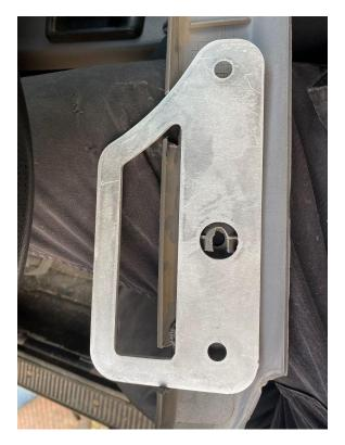
6. MAKE SURE TO FINISH PARACORD BEFORE REINSTALLING MOUNTS. Once your trimming is complete install the mounts and reinstall the trim. (Your factory screws should be long enough if installed correctly but we have provided longer screws and self tappers if needed.)
