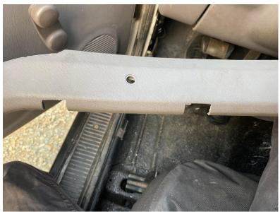
5. You may need to also cut part of the plastic around the mounting hole on the back side of the trim to allow the mounts to sit more flush inside of the cutout.
