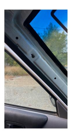
2. Once the holes are located drill them out to a ½ hole using either a step bit or multiple drill bits to ensure a clean precise hole. Insert the Riv Nuts into these holes (tapping with a small hammer may help). Using a Nut Sert tool, rivet the Nuts into the A Pillar.
