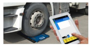
In the example, an application with wireless platform, WWSDUAL option, analogue platform, Bluetooth BLTH and DINI SMART AXLE weighing App, that can be downloaded from the Playstore at the link below:
