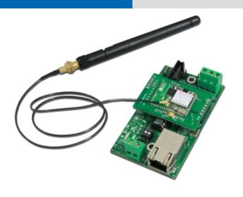
Small size, excellent signal quality and adjustment of the antenna's inclination and orientation, are just a few features of this product which allow for an easy wireless connection of any scale or weighing system to the company's computer system; it' easy to install and it's fitted with a cable for the connection to the indicators. The module does not exclude the use of other Dini Argeo products on the system, such as Control Light, Alibi Memory, attached or external printer.
