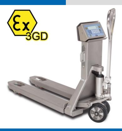
Pallet truck scales, with built-in electronic weighing, suitable for harsh working conditions and dangerous areas classified as hazardous (ZONE 2, 22) in accordance with Ex II 3GD IIC T6 T130°C X protection. The weight detection made with four Atex certified IP68 stainless steel load cells guarantees the precision in all work conditions. Structure entirely in stainless steel. Available also CE-M APPROVED.
