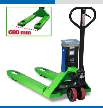
Pallet truck scale, with built-in electronic weighing, fitted with forks 680mm width, which making it ideal for the handling of pallets in the Food & Chemical Industry Sector. Fitted with rechargeable extractable battery. Available also with a built-in printer as well as CE-M DOUBLE RANGE approved.
