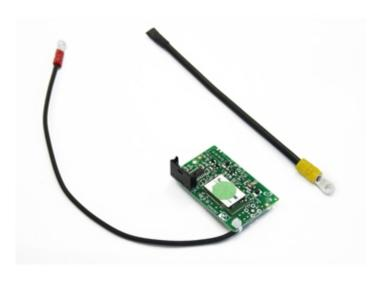
Interface which allows to convert a RS232 signal into an 868MHz radio frequency. Up to 50 transmission channels, configurable through the programme for PC. Thanks to the reduced energy consumption and to the long transmission distance, this is ideal for creating mobile systems or wireless radio transmissions.
