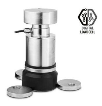
Digital compression load cells, C4 precision class, with IP68 protection. Ideal for approved CE-M weighbridges or silos and tanks. Fitted with self-aligned articulated joints, self centering plates and protection washer for an excellent installation.
