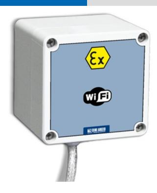
WIFI module for the wireless data communication in ATEX 2 and 22 zones, with protection methods according to: ATEX II 3G Ex nA IIB T6 Gc X for gases ATEX II 3D Ex tc IIIC T125°C Dc IP66 X for dust. It can be applied to both bench/floor scales as weel as mobile scales, such as pallet truck scales or pallet weighing scales. It allows the easy wireless connection to the company computer system and the data transmission at a very long distance.
