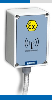
Radio frequency module for the wireless data communication in ATEX 2 and 22 zones, with protection methods according to: ATEX II 3G Ex nA IIC T6 Gc X for gases ATEX II 3D Ex tc IIIC T125°C Dc IP66 X for dust. It can be applied to both bench/floor scales as weel as mobile scales, such as pallet truck scales or pallet weighing scales, and it allows to transmit data at a very long distance.
