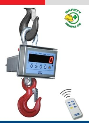
Stainless steel crane scales, with large 40mm DOT LED display, for maximum visibility from any angle and in any light condition, also with direct sunlight. Sturdy and reliable, usable in any environment, inside or outside. Minimum reduction of the lifting space of the crane. IP67 protection, from dust and rain. Available also CE-M APPROVED. Fitted with test certificate obtained with sample weights.
