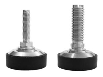
Stainless steel articulated feet designed in order to obtain the best weighing performances, particularly suitable for creating scales with 4 load cells. Extremely compact and easy to install, the feet minimize the height of the platform and ensure a perfect decoupling of the lateral forces during the weighing operation.
