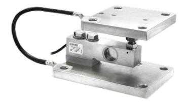
Assembly kits for SB... shear beam load cells: accessories suitable for weighing hoppers, tanks, platforms, etc. The special articulation guarantees an excellent measuring accuracy also in the presence of dilatations and/or bending of the weighing structure. Furthermore it's possible to adjust the height for an optimal levelling of the structure to be weighed.
