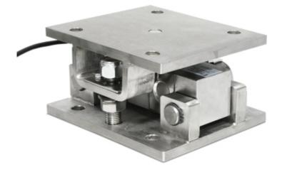
Mounting kits for DSBi double shear beam load cells: Accessories suitable for weighing hoppers, tanks, platforms, etc. etc. The special articulation guarantees an excellent measuring accuracy also in the presence of dilatations and/or bending of the weighing structure.
