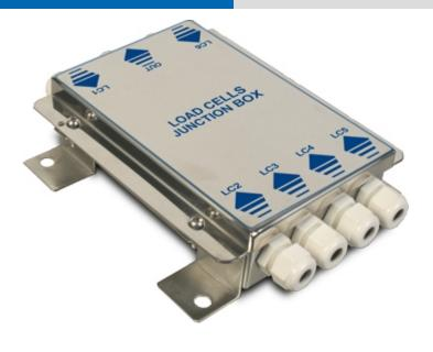
Stainless steel junction box with IP65 protection from water and dust, and fitted with electronic board for junction and equalisation of 4 or 6 load cells. Terminal board with screw for easing the connection of the load cells and the signal adjustment trimmer, for an accurate and reliable equalisation.
