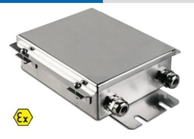
Stainless steel junction box with IP66 protection from water and dust, and fitted with an intrinsically safe electronic board for junction and equalisation of load cells. Terminal boards with screws for easing th connection of the load cells and signal adjustment trimmer, for an accurate and reliable equalisation. Marking: ATEX II 2G Ex ib IIC T6 Gb for gases. ATEX II 2D Ex tb IIIC T115°C Db IP65 for dust.
